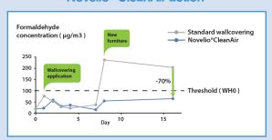
laboratory and in normal conditions with same results: **70% absorption, permanently captured** <sup>(3)</sup>. A benchmark study was made in a room of a French nursery:
